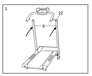
Push the Wire Harness (22) into the right Upright (6) as you insert the Handrail (16) into the right and left Uprights (6). Be careful not to pinch the Wire Harness. Tighten a Handrail Bolt (12) with a Washer (11) into each Upright.
